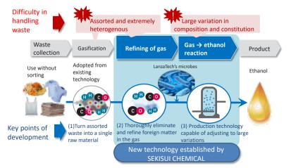
To produce ethanol from garbage, the first thing vou have to do is to make garbage burn by itself in a state of low oxygen, resolve it into a molecular level and convert it into gas. Because most of this gas turns into carbon monoxide and hydrogen, ethanol is produced by causing microorganisms that like this environment to metabolize it.
