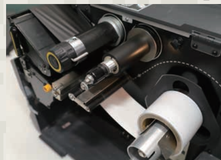
Inside of a thermal transfer printer. The white roll in the foreground is label material, and the black roll in the upper left is the ink ribbon. Both are heat resistant, preventing the ink from burning off even when exposed to high temperatures.
