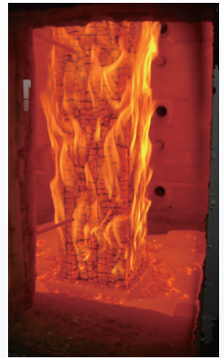
COOL WOOD offers a level of fire resistance that has even passed a three-hour fire resistance test.
