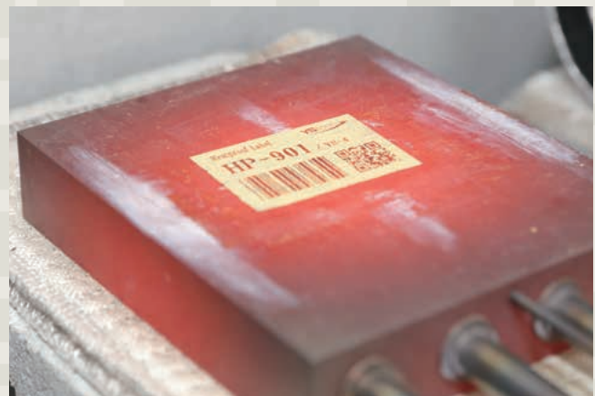
Heat resistant barcode labels can be applied directly to high-temperature materials, enabling consistent control during heat treatment processes.
