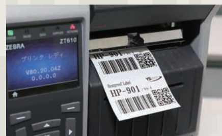
HEATPROOF barcode labels can be printed on commercial thermal transfer printers.
