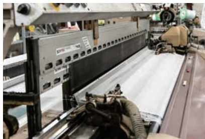
Above: Process of winding the warp threads for the weaving machine. 10,000 warp threads are needed for a single piece of fabric.
