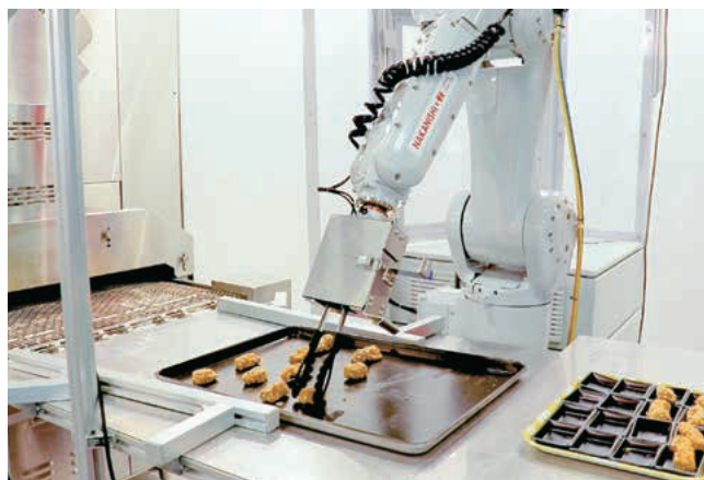
Placing fried chicken in individual containers. There’s no need to rewrite the program for different sizes and dimensions, even when grasping soft foods.
