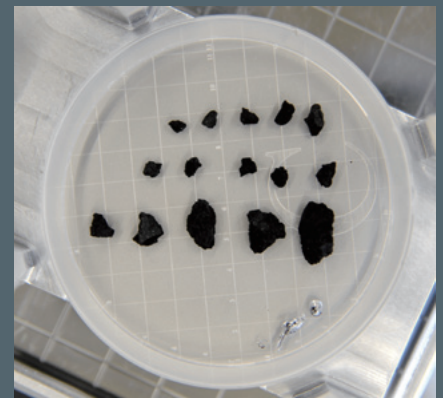
Rock and sand samples brought back by Hayabusa2 from the asteroid Ryugu. The largest specimen exceeds 10mm. The diameter of the Petri dish is 60mm and the grid spacing is 5mm.
