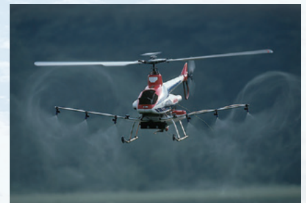
An unmanned helicopter sprays agricultural chemicals evenly over rice paddies.
